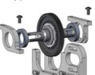
This will locate the bulkheads over the correct holes in the chassis to fasten the bulkheads using 5252 or 5262 screws. Be sure to also align the CVD's into the outdrives.
